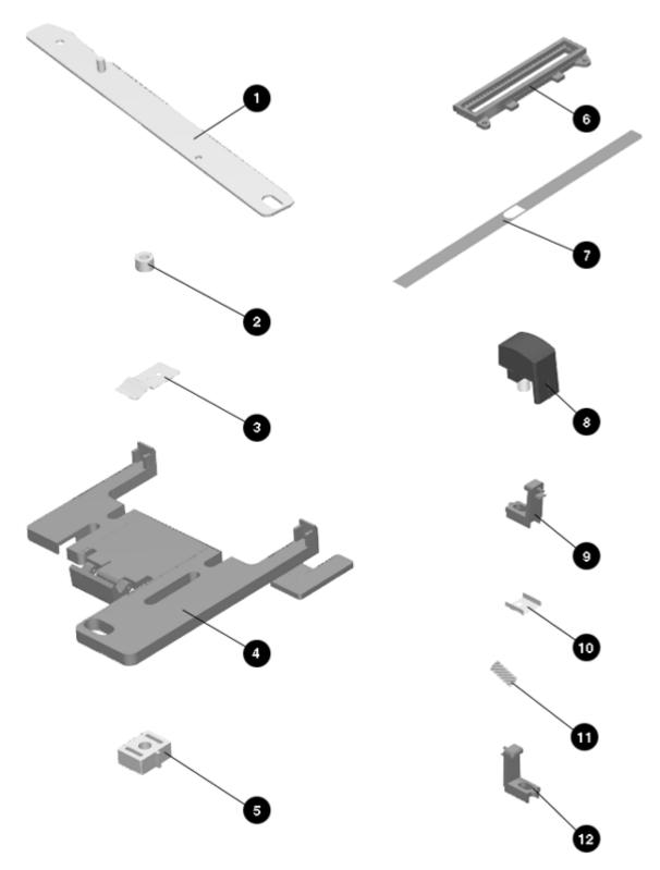
Figure 3-14. MultiBay and MultiBay-ISA Expansion Base Mechanical Kit
